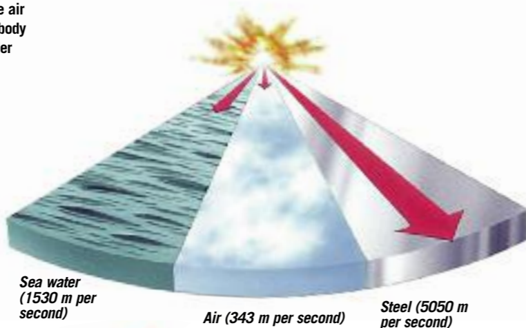
The speed of sound varies depending on the substance it travels through. Atoms in steel are closer than molecules in air, so the vibrations of sound move faster and further.
